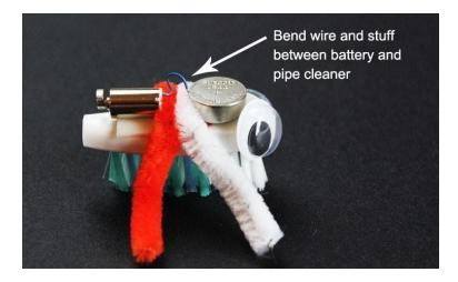
Try experimenting with different variations of construction including using bigger motors and bigger brushes.
