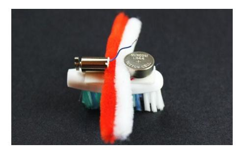
Bend the pipe cleaner legs down and around the toothbrush head.
